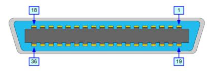
Figure 3-6, Parallel Connector Pin Assignments
